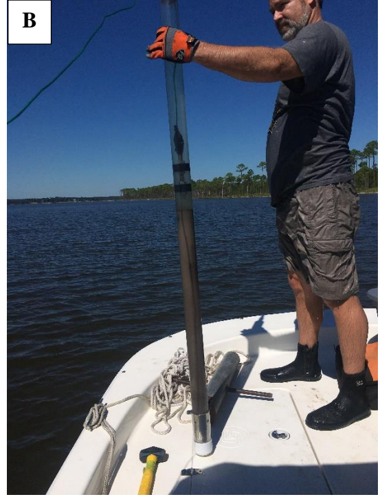
Figure 4.3 Gravity coring device in use at Bon Secour Bay (A) and Perdido Bay (B).
