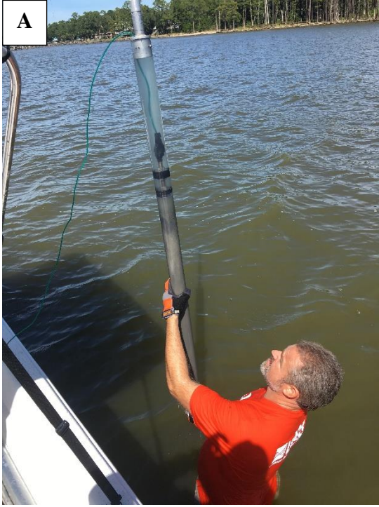
Figure 4.3 Gravity coring device in use at Bon Secour Bay (A) and Perdido Bay (B).
