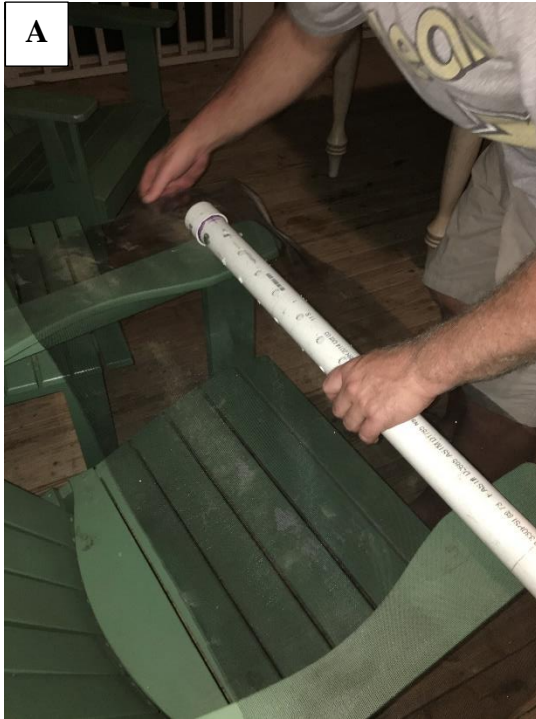
Figure 4.7 Piezometer construction and installation.
