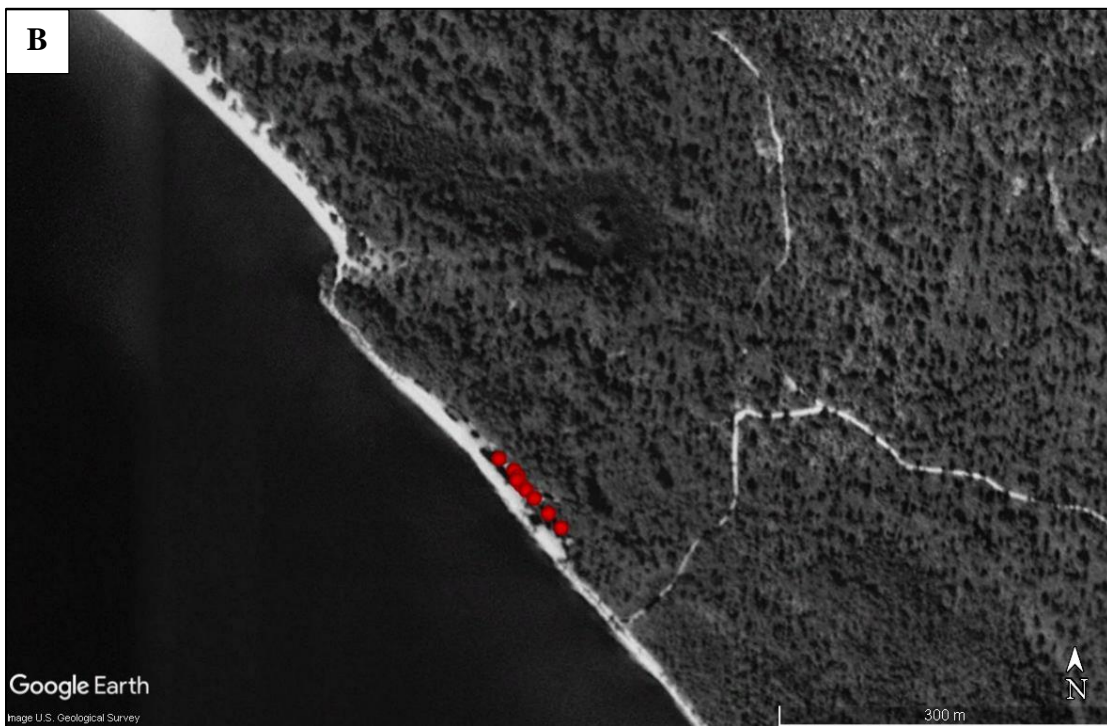
Figure 4.1 Comparison of historical shoreline imagery (Google, 2019) overlain by recent high-tide shoreline GPS points (red dots) surveyed in October 2018. (A) Bon Secour Bay site image from 1992, B) Perdido Bay site image from 1994.
