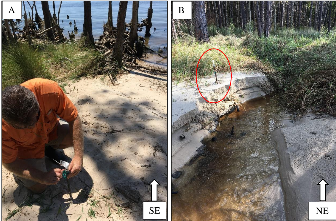
Figure 5.22 A) Erosion pin 1 in May 2018. B) Erosion pin 1 (circled in red) in November 2018.
