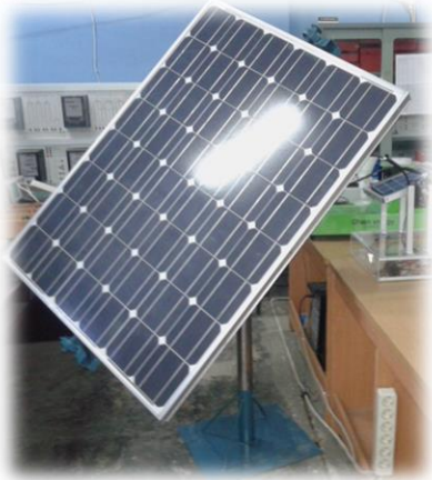
Figure 10. Solar Tracker construction of 180 Wp solar panel
