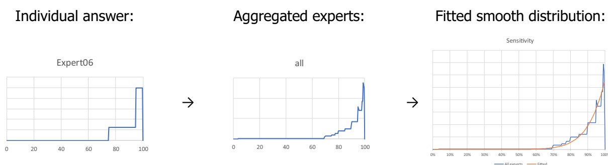
Figure 2: Process of fitting of a Beta-distribution to smooth the outcome
