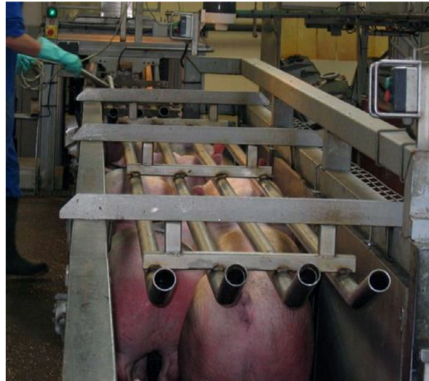
Figure 13: Pigs being forced in a single line raceway to enter the automated electrical stunning method (Source: Virginie Michel)
