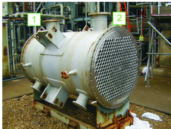
Figure 2.12 – Tubular reactor (steam inlet at point 1 and outlet at point 2).
