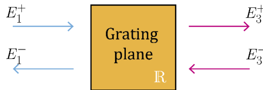
Figure 4. Propagation in one dimension from an incoming and outgoing plane wave on a grating plane, related to the transfer matrix \mathbb{R} .
