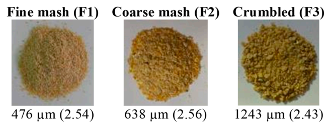
Figure 2. Images of the feed types used in the experiment with their respective geometric mean diameter and geometric standard deviation (between parentheses) [11].
