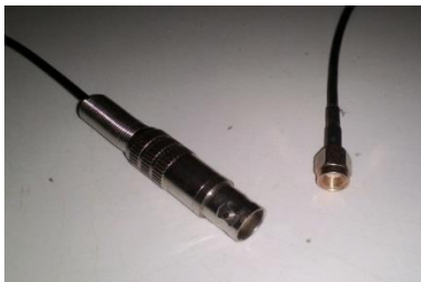
Gambar 8 Pigtail NBC male to RP-SMA female
