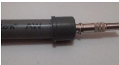
Gambar 9 Pemasangan Cover antenna
