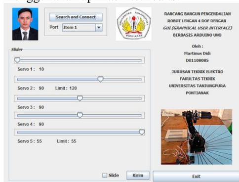
**Gambar 3.16** Tampilan Interface Pengendali Robot Lengan 4 DOF.
