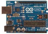
Gambar 2.2. Board Arduino Uno
