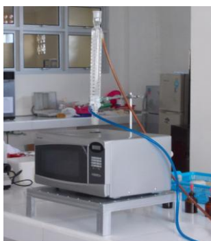
Figure 1. Modified microwave extractor
