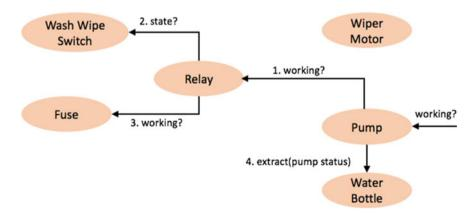
Fig. 4.4 Collaborations between the objects for wash operation
