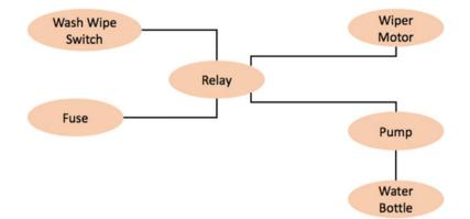
Fig. 4.5 Wash-wipe system structure
