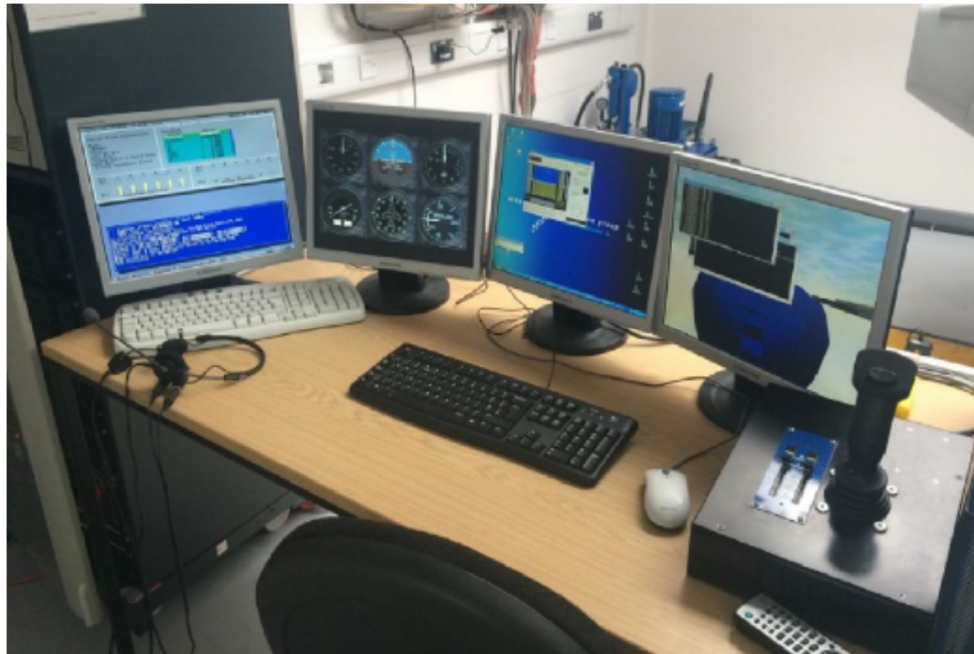
Figure 7. Engineering flight simulator instructor station
