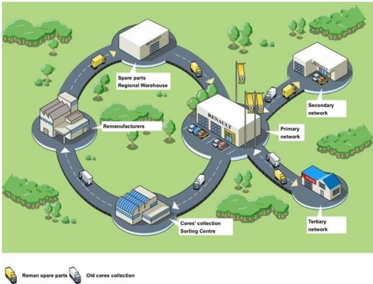
Figure 3-15: Reverse logistic network employed in Choisy-le-roy plant of Renault; from Ellen MacArthur Foundation made (2012).
