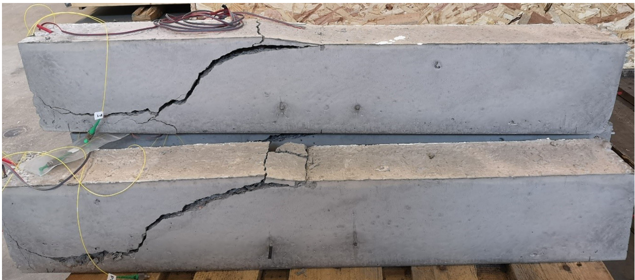
Figure 3. Beam specimens after testing displaying the developed shear failure mechanism.
