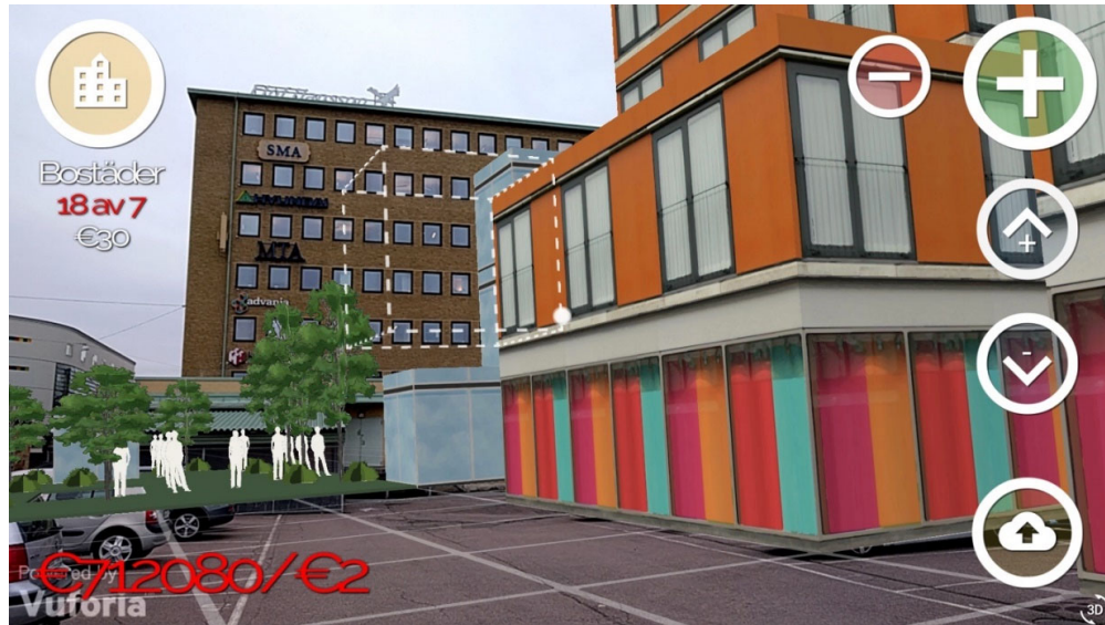
Figure 10. User interface for choosing an urban function on top left of the screen, addition and deletion buttons are on the top right. The two middle buttons indicate up or down, i.e., if to build on top of or below the selected box. The button at the bottom right indicates an upload function. The text and the numbers on the top left indicate the currently chosen urban function, available and used number of blocks, and the cost of one block of the chosen function. The numbers at the bottom left indicate available funding and remaining funding.
