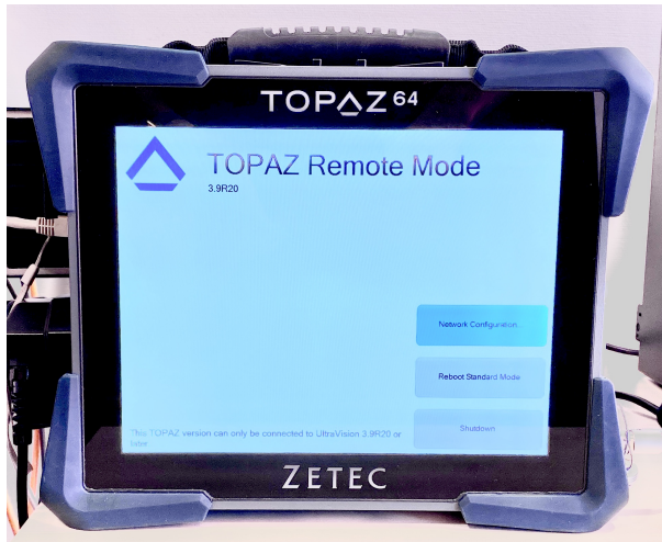
Figure 4.1: Data acquisition hardware unit, TOPAZ64
