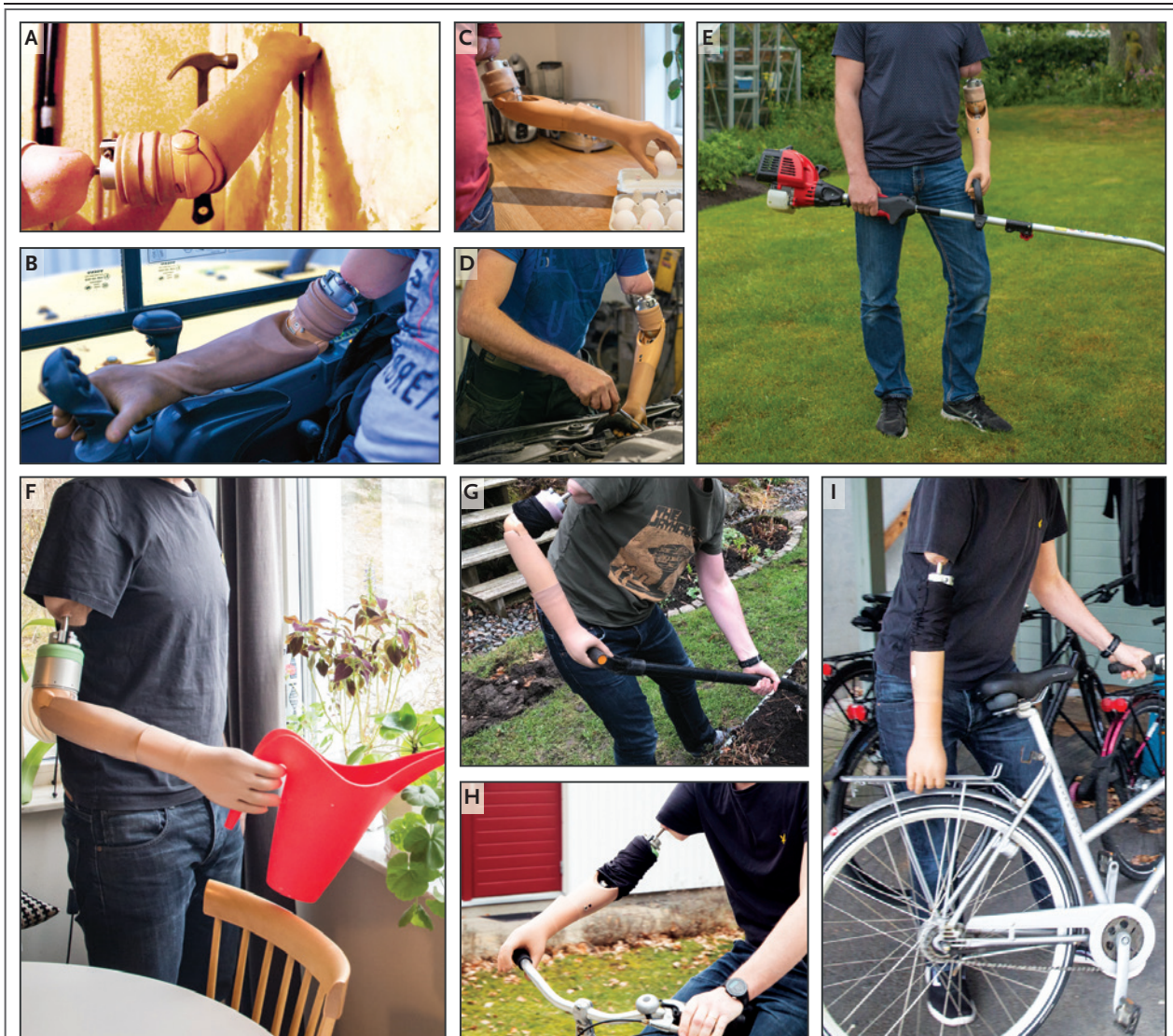
Figure 2. Neuromusculoskeletal Arm Prosthesis Used Unsupervised in Daily Life.
