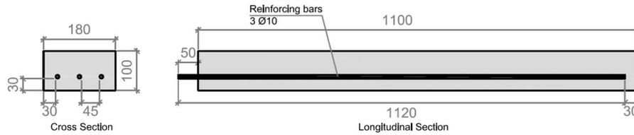
**Fig. 1** Specimen geometry
