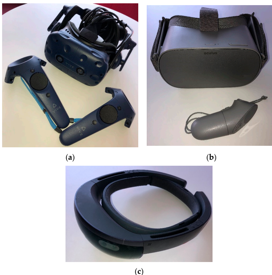
Figure 7. Images of the virtual reality and augmented reality headsets. (a) illustrates the VIVE headset and controllers, (b) shows the Oculus headset and controller with (c) depicting the Hololens.
