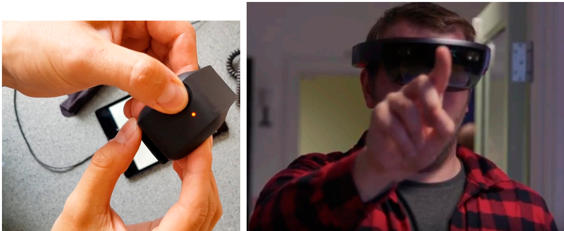
Figure 5. Shows the Empatica E4 heart rate and galvanic skin response (GSR) sensor ( Left ) and augmented reality solution ( Right ).
