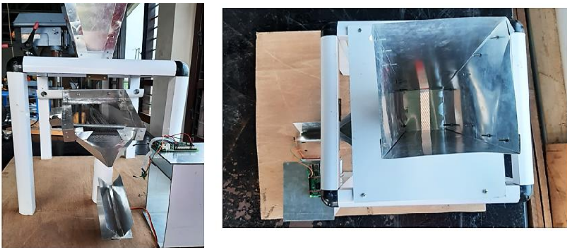
Figure 4.2: The fabricated cowpea sorter system
