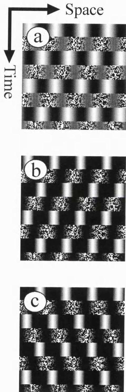
Figure 7.1: (a) Space-time plot showing an interleaved luminance/contrast modulation stimulus. The results of halfwave rectification around mean luminance are shown in (b) and (c) with: (b) values above mean luminance and (c) values below mean luminance.
