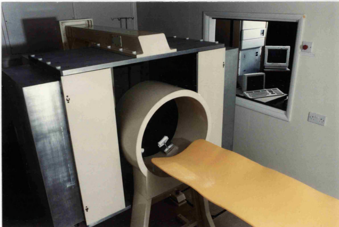
Figure 6.1: MUP-PET positron camera : the two detectors rotate through 180° about the patient couch.
