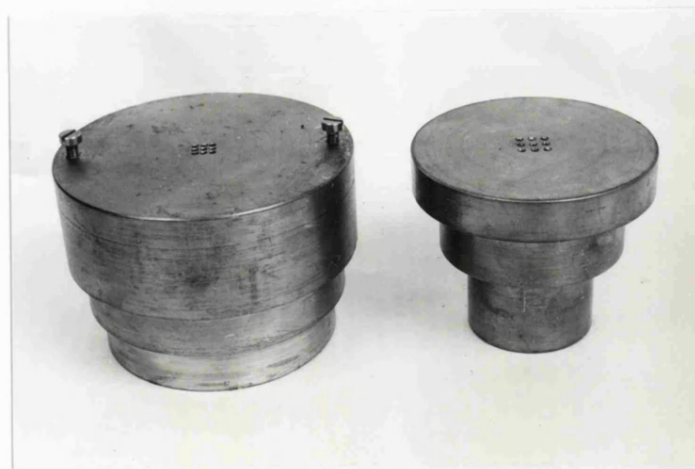
Figure 5.3: Pair of nine-hole 3mm diameter parallel-bore collimators.
