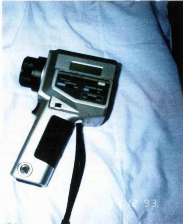
Plate 4.5.2-IIa : Minolta luminance meter
