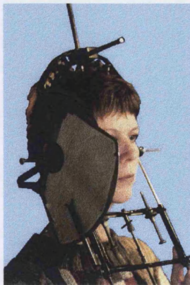
Figure 1: A Prosthometer which measures head size and the position of the teeth relative to the head
