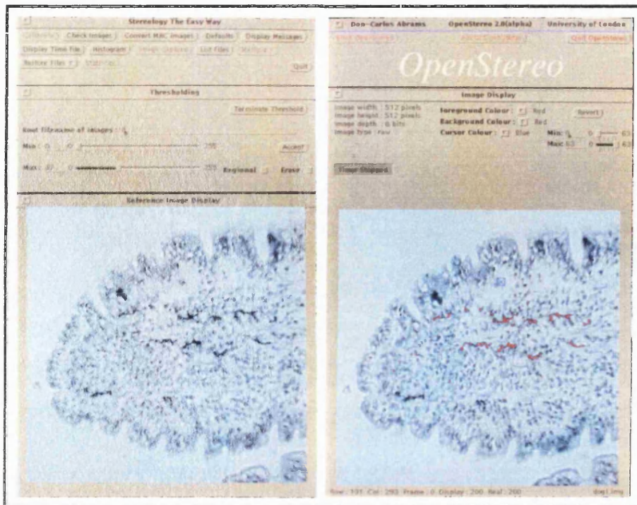
Fig 113: Thresholding of captured images using OpenStereo
