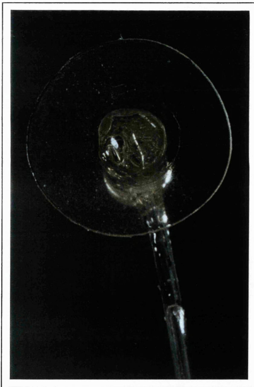
Fig 26: Photograph illustrating the single fibre laser Doppler probe
