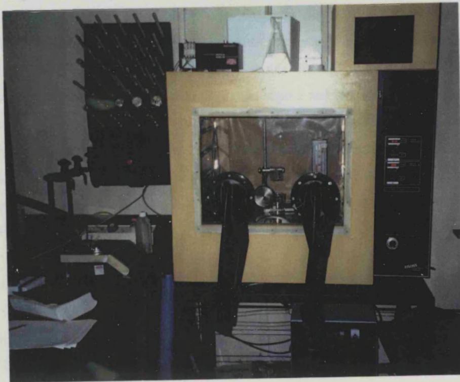
Figure 4.1: Modified (in-house built) humidity chamber
