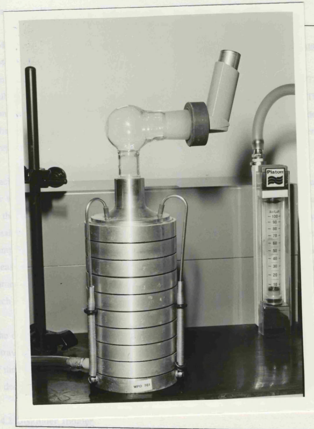
Figure 3.3 The Andersen Cascade Impactor.
