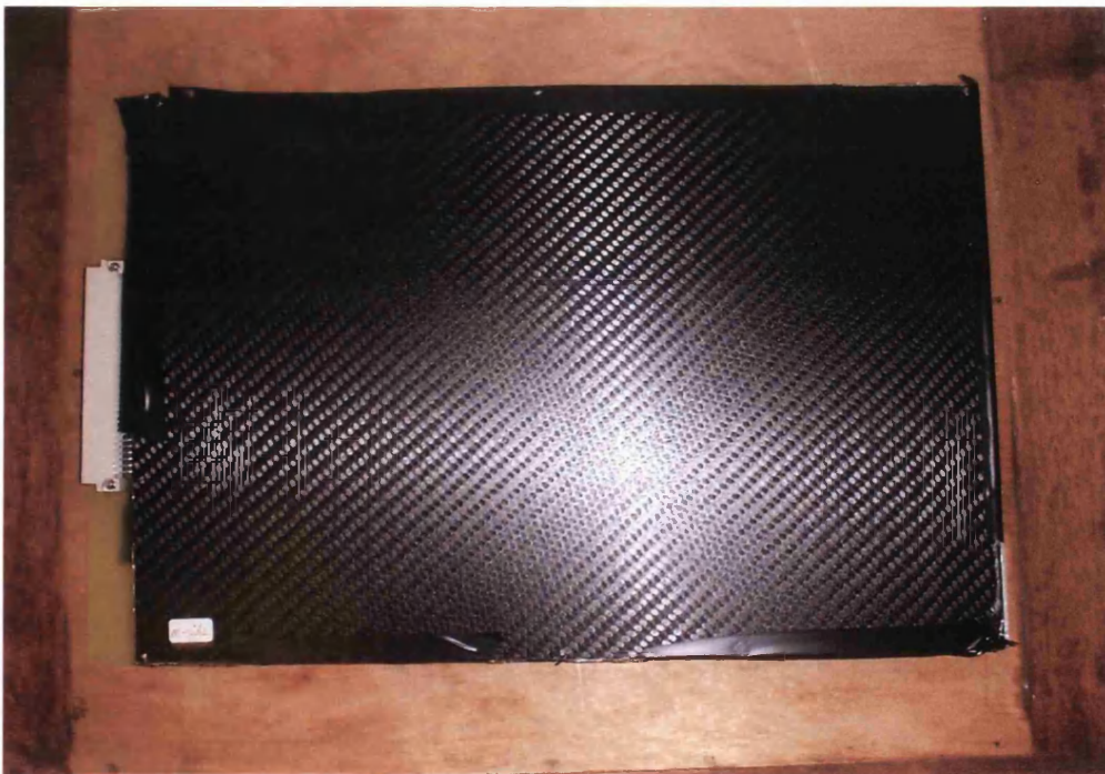
Fig. 5.2: Photograph of a detector plane (the carbon fibre cover was here removed).
