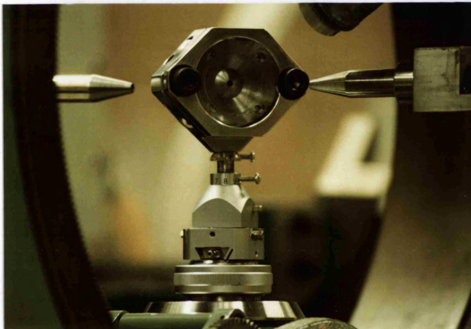
Figure 2.6: a) Photograph of the Picker four-circle diffractometer used for all the X-ray diffraction experiments located inside a radiation enclosure; b) a close-up of the modified goniometer head supporting a DXR4-type DAC.
