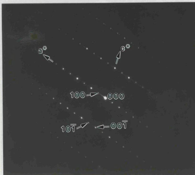
Figure 2.15: a) Bright field TEM photograph of a typical area of an FeSiO 3 clinoferrosilite crystal used as the starting material for the high-pressure experiments described in Chapter 5. The contrast is probably due to strains associated with the formation of antiphase domains occurring upon pressure release as a result of the C2/c → P2 1 /c transition (see Chapter 5 for details); b) the corresponding diffraction pattern, showing some streaking of the reflections along a* due to the stacking disorder.
