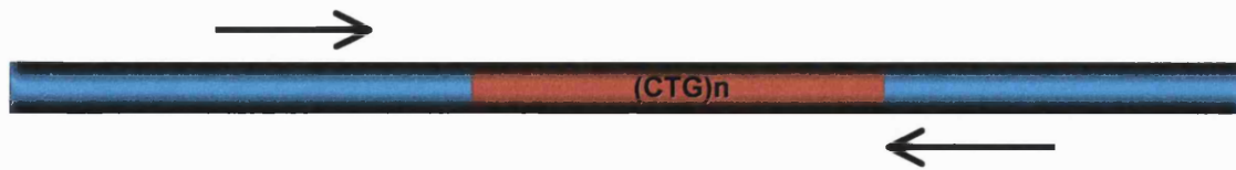
Figure 4.1 DM primers (arrows) mapped to the CTG repeat region within exon 15 of the DMPK gene. By measuring the amplified fragment size, the copy number of the CTG repeat can be calculated.
