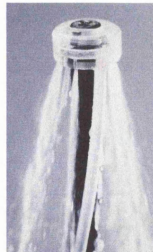
Figure 8.1 Water jetting out of the spray head lifts an endoscope vertically upwards.
