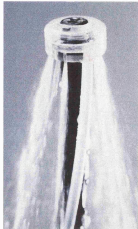
Figure 4.12. Acrylic head with two external supply tubes. The photo shows a paediatric endoscope being pulled vertically upwards.
