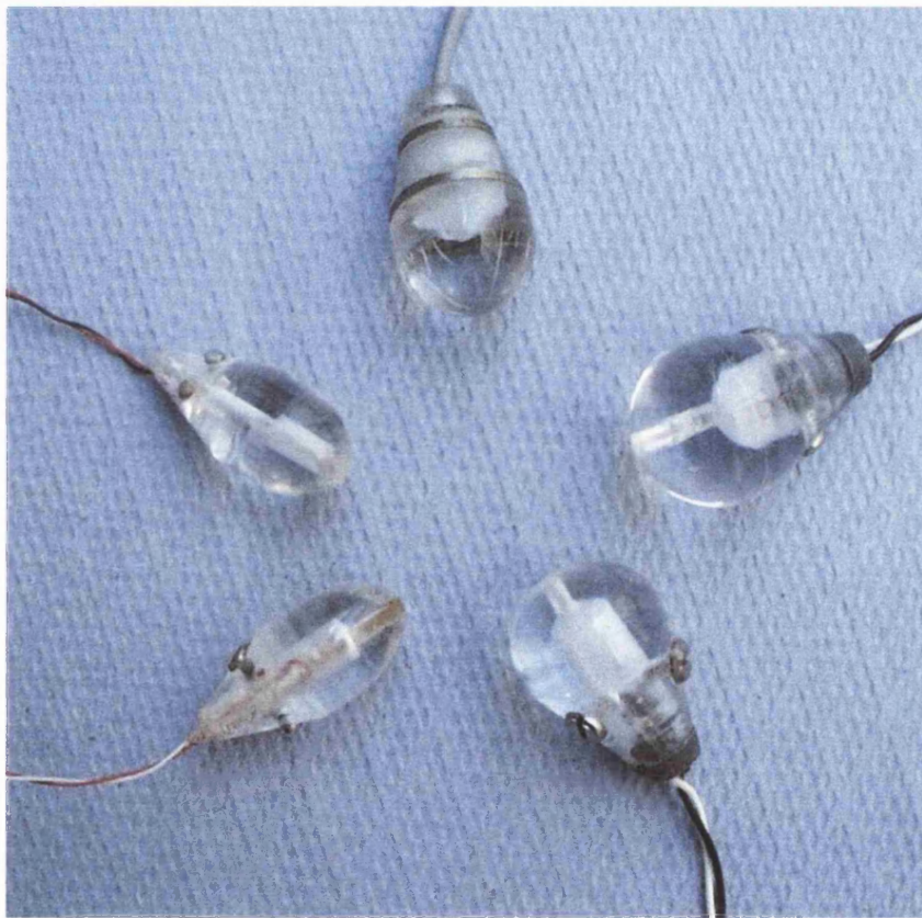
Figure 6.9 Devices for stimulating contractions of the colon. Device E1 is at 12 o'clock, Device E2 at 2 o'clock, etc.
