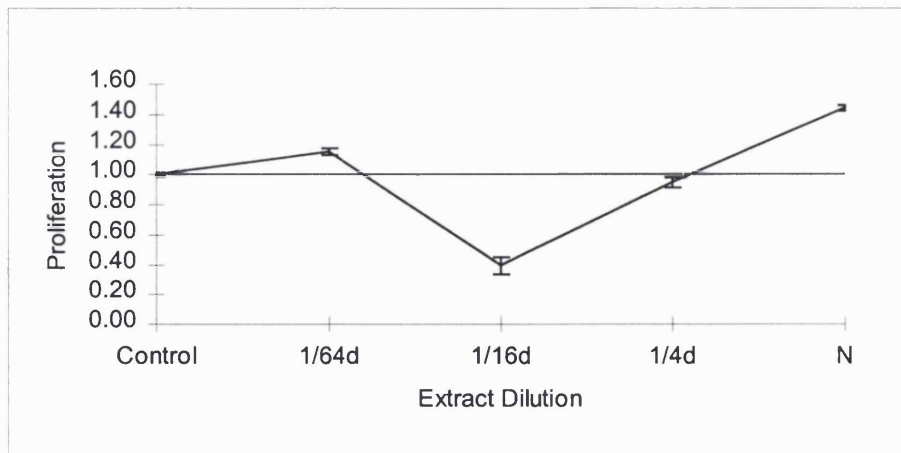
Figure 137: MTT test result for glass \text{Ca}_{32}\text{Na}_{23}\text{P}_{45} (test result after 2 days of incubation)
