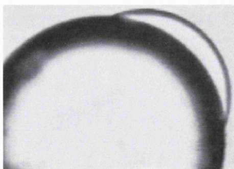
Figure 6-37 Receding contact angle of silicone oil on glass ballotini in a solution of SDS 10^{-3} M. Only the ballotini has been left to equilibrate for 15 minutes in the bulk medium before the contact takes place. The receding angle is 27.1 deg.
