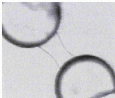
Figure 6-38 Configuration of maximum liquid bridge strength. Glass ballotini of \sim 50 \mu\text{m} diameter are held together by a silicone oil liquid bridge in a solution of 10^{-5} M CTAB and 10^{-3} M NaCl.
