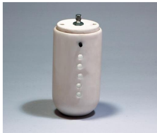
Figure 11: The PTC recording system was made to be small enough to be handheld and simple to operate and record data points. The electronics were secured in a 3D printed plastic case.
