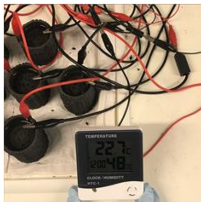
Figure 3. Demonstration of powering a digital weather station with additive manufacturing (AM)-built MFCs.
