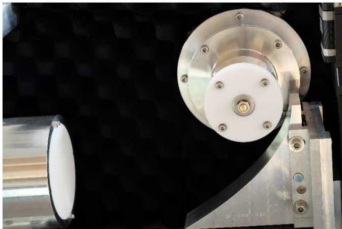
Fig. 1. Photo of the mode generator setup with the lens system, the quasi-parabolic mirror and the mode generator cavity.
