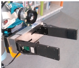
Fig. 4: Gripper fingers equipped with force/tactile sensors.
