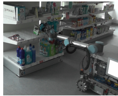
Fig. 2: Mobile manipulator used in the experiments.
