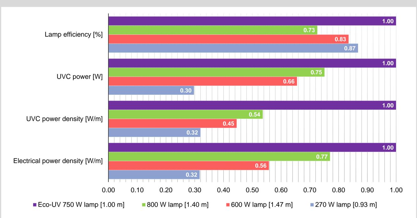
The developed lamp was compared with three commercial lamps in terms of efficiency, UVC output power level, UVC output power density and input electrical power density. The figure shows the normalized values for the comparison.
