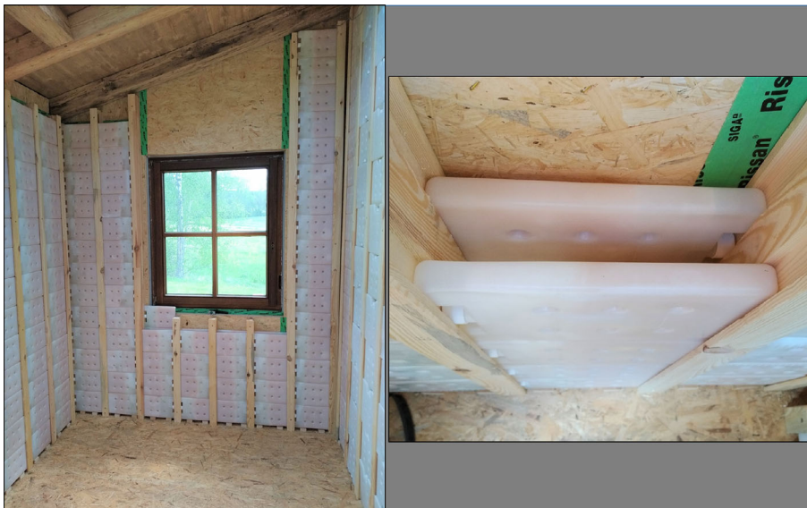
FIGURE 2 Two-layer integration of the phase change material (PCM) boxes in the test-room [Colour figure can be viewed at wileyonlinelibrary.com ] [Colour figure can be viewed at wileyonlinelibrary.com ]
