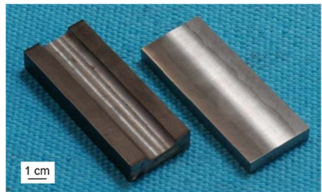
Fig. 5 MVT specimens before deposition of weld metal (left) and after finishing, ready to test (right)
