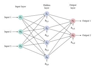
Figure 4.1: Visualization of an MLP. For better clarity, the bias terms are left out.
