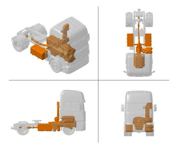
Figure 22: CAD model of current conventional HDV tractor that complies with German road traffic regulations (Jadim, 2018)
