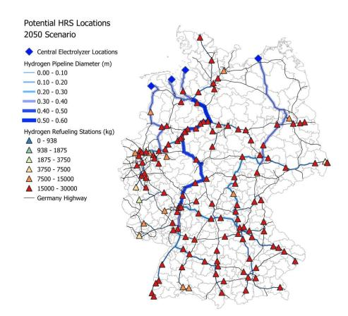
Figure 33: Pipeline network to supply the HDV-HRS network from the reference scenario with hydrogen
