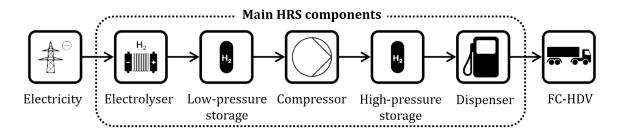
Figure 24: Schematic structure of a HRS and its main components (power supply, electrolyzer, LP-storage, compressor, HP-storage, dispenser and end-user) (Grüger, 2017)<sup>36</sup>
