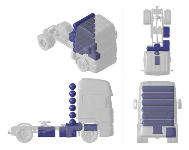
Figure 23: CAD model of potential FC-HDV tractor after replacing the diesel engine with a fuel cell powertrain, which meets user and legal requirements
