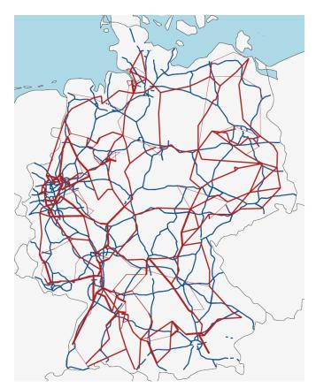
Figure 40: Overlay of German highway network (blue lines) and stylized high-voltage transmission electricity network (red lines)
