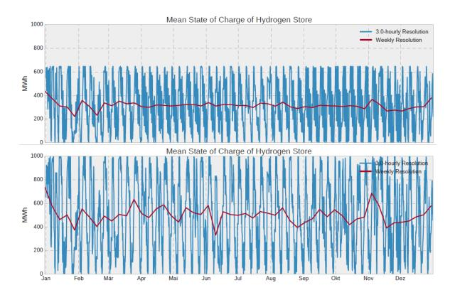
Figure 48: Mean state of charge of LP hydrogen storages at the HRS for scenario A (top) and scenario B (bottom)
