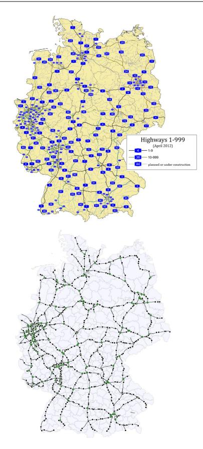
Figure 12: Top: German highway network of 121 highways, about 13,000 km and 2,500 nodes (Weltkarte.com, 2012); bottom: highway network arcs (black lines), nodes (black dots) and junctions (green dots)
