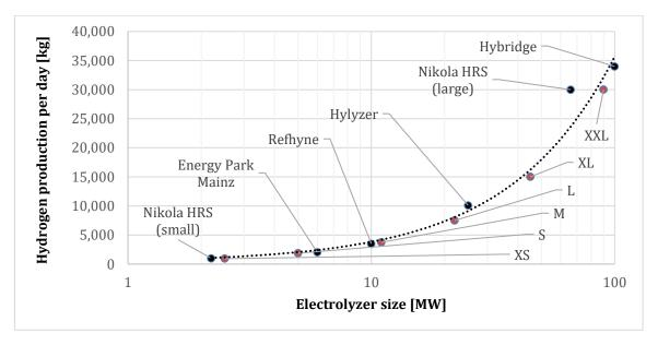
Figure 26: Examples of PEM electrolysis projects announced by capacity (in MW) and daily hydrogen production (in kilogram hydrogen per day) and the potential electrolyzer sizes for HDV-HRS portfolio.<sup>49</sup>
