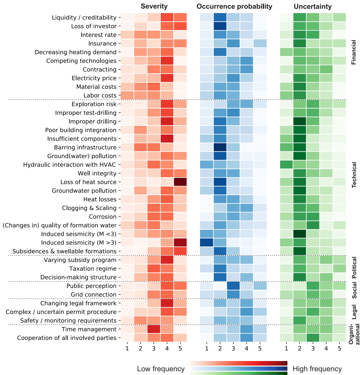
Figure 4.7: Relative frequencies of the risk item ratings grouped by the severity, occurrence probability and uncertainty.
