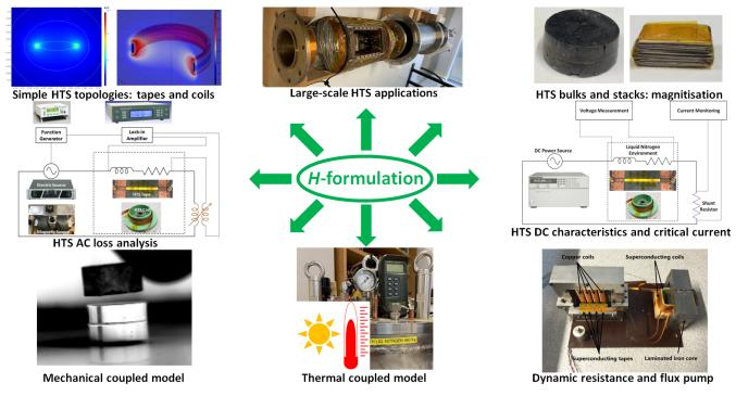
FIGURE 1. Scope of the applications of H-formulation: AC loss calculation, critical current and DC characteristics, HTS bulks and stacks magnetization, large-scale HTS applications, electromagnetic-thermal and electromagnetic-mechanical coupled problems, dynamic resistance and flux pump.
