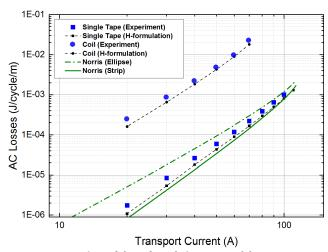
FIGURE 2. Comparison of the *H*-formulation FEM model, measurement, and analytical solutions (Norris ellipse and Norris strip), for the analysis of the AC loss from a HTS a single tape and double pancake coil, with transport current at 50 Hz, with data from [56].
