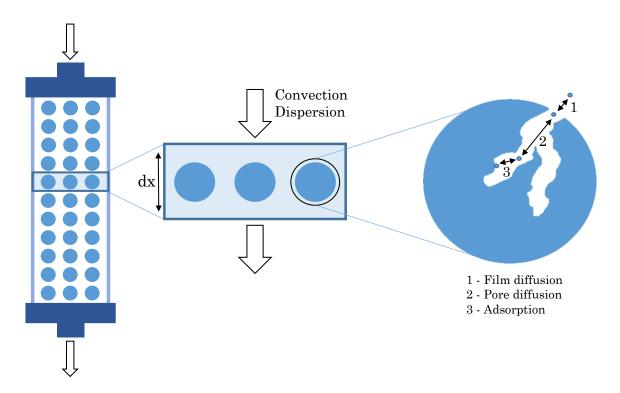
Figure 1.4: Processes in chromatographic columns, which can be modeled by setting up differential mass balances. Not included in the figure is surface diffusion, which can also contribute to mass transfer inside the pores. Figure adapted from Seidel-Morgenstern et al.<sup>94</sup>.
