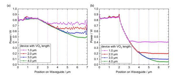
**Figure 7.6:** Simulated optical power flow of the TE mode along the propagation direction of the type 1 device with an air cladding at (a)  $T < T_{tr}$  and (b) at  $T > T_{tr}$ . Different colors indicate devices with VO<sub>2</sub> structures having different lengths. The position of the beginning and the end of VO<sub>2</sub> structures are indicated by dashed lines.
