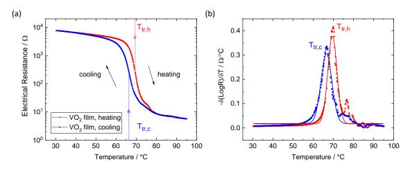
**Figure 6.1:** (a) Electrical resistance of a VO<sub>2</sub> film as a function of temperature. The phase transformation temperatures upon heating  $T_{tr,h} = 69.5$  °C and cooling  $T_{tr,c} = 66.4$  °C are indicated with red and blue arrows, respectively. (b) Transition temperatures are determined by the maximum of Gaussian fit of the first derivative of electrical resistance characteristics. Adapted from [133].
