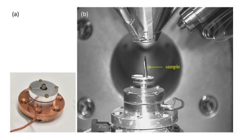
**Figure 6.11:** (a) Micro heating-cooling stage (MHCS) for the homogenous temperature control of samples inside a SEM. (b) Side-view to the SEM chamber. The sample is fixed at an angle of 80 ° to the MHCS, which is connected via an integrated vacuum/air splitter in the chamber flange to a temperature control unit.
