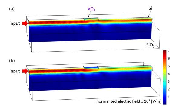
**Figure 7.4:** FEM simulation of the normalized electrical field for the TE mode. The VO<sub>2</sub> structure on top of the waveguide has a length of 0.8  $\mu$ m and a thickness of 50 nm. (a) The VO<sub>2</sub> is in insulator state (T < T<sub>tr</sub>) and nearly the entire light is transmitted to the output. (b) The input light is largely absorbed by the VO<sub>2</sub> in metal state (T > T<sub>tr</sub>).
