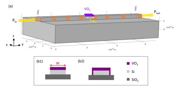
**Figure 7.3:** (a) Three-dimensional (3D) FEM simulation model of a Si waveguide switch including a VO<sub>2</sub> film covering a Si waveguide on a SiO<sub>2</sub> substrate. The representative power integral surfaces along the waveguide are indicated by orange rectangulars. (b1) and (b2) depict schematic cross-sections of type 1 and type 2 devices, respectively. The length and width of the VO<sub>2</sub> structure are indicated by  $l_{VO_2}$  and w, respectively.
