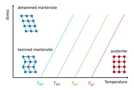
**Figure 2.1:** Schematic stress-temperature phase diagram of a SMA. The shape change associated with the phase transformation for a single crystal with six unit-cells is illustrated.  $T_{Mf}$  and  $T_{Ms}$  are the martensitic finish and start temperatures, respectively.  $T_{As}$  and  $T_{Af}$  indicate the austenite start and finish temperatures, respectively. Adapted from [53].
