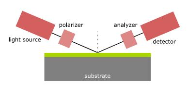
**Figure 4.5:** Schematic of a basic setup of an ellipsometer. Optical constants and the thickness of the film (indicated in green) is determined through measurement of change in the polarization of the incident light after interaction with the material.
