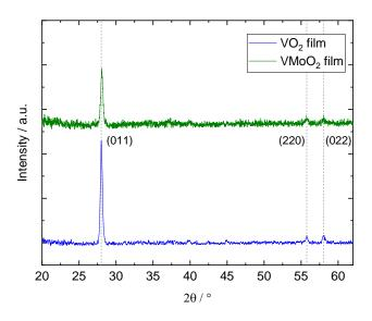
**Figure 5.1:** XRD patterns of VO<sub>2</sub> and VMoO<sub>2</sub> films. Peaks at  $2\theta = 28^{\circ}$ , 55.6° and 57.7° correspond to the (011), (220) and (022) crystal-plane orientations of the monoclinic phase M1, respectively. Adapted from [133].
