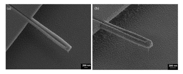
**Figure 5.4:** (a) Top-view and (b) side-view scanning electron micrographs of a free-standing double-beam fabricated by the deposition of a 100-nm thick  $VO_2$  film on the pre-structured SOI substrates.
