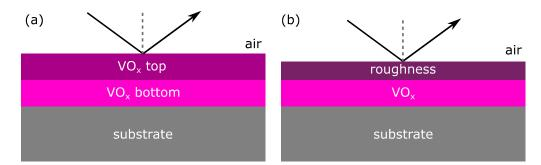
**Figure A.1:** Ellipsometry models of VO<sub>2</sub>-based films. (a) A two-layer model including layers based on Tauc-Lorentz dielectric materials. (b) A one-layer model having a roughness based on EMA.
