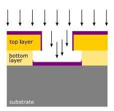
**Figure 4.3:** Sketch of the cross section of a substrate with a coating of PMMA bilayer after deposition. Material will be deposited on surfaces and sidewalls of the top layer. The undercut profile largely prevents the deposition on sidewalls of the bottom layer and below the top layer, providing a region for the contact with acetone in the lift-off process.
