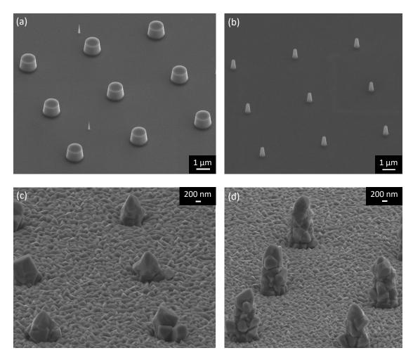
**Figure 5.8:** Scanning electron micrographs of (a) Si pillars with diameters of  $d = 1 \ \mu m$  and (b) Si nanopillars with  $d = 100 \ nm$ . Through deposition from top, (c) VO<sub>2</sub> single crystals grow on top of Si nanopillars. (d) Oligocrystalline-like structures are realized for a longer time of the deposition. Crystal growth on Si nanopillars with  $d = 100 \ nm$  results in large grains having diameters of around 500 nm.
