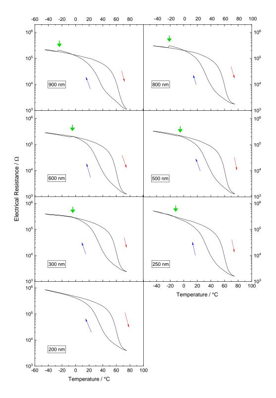
**Figure 6.4:** Electrical resistance as a function of temperature for VMoO<sub>2</sub> nanobridges with widths w = 200 to 900 nm, having the same length of  $l = 5 \mu m$ . The metal to semiconductor (R-M) transformation persists for the nanostructures. The change of the electrical resistance due to the M2-M1 phase transformation is indicated by green arrows. Adapted from [133].
