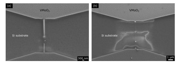
**Figure 6.5:** Scanning electron micrographs of VMoO<sub>2</sub> nanobridges with widths of w = 100 nm and lengths of  $l = 5 \mu m$  after failed electrical measurements. (a) Local overheating leads to damaging of the nanobridge due to the less dense structure of film grains, and, (b) instabilities in the electrical current results in melting of the entire nanobridge.
