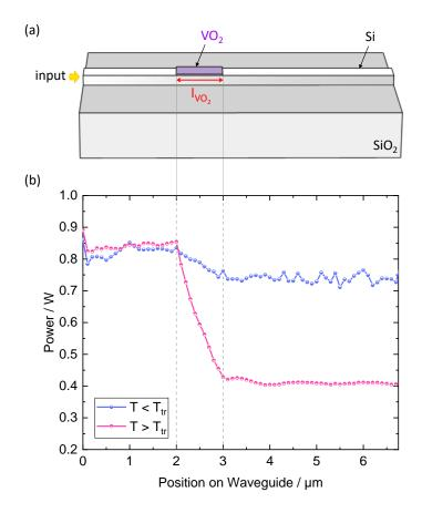
**Figure 7.5:** (a) Geometry illustration of the photonic device type 1 with air cladding. The VO<sub>2</sub> structure on top of Si has a length of  $l_{VO_2} = 1 \ \mu m$  and a thickness of 30 nm. (b) Power profile of the TE mode along the propagation direction in insulator state  $T < T_{tr}$  and in metal state  $T > T_{tr}$ . The position at the beginning and the end of the VO<sub>2</sub> structure is indicated by dashed lines.
