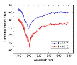
**Figure 7.14:** Transmitted power intensity of a type 1 device operating with TM mode. The VO<sub>2</sub> structures has a thickness of 40 nm and a length of  $l_{VO_2} = 4 \ \mu m$ . After heating of the sample from 20 to 80 °C, the transmission decreases.
