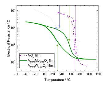
**Figure 6.2:** Electrical resistance as a function of temperature for a VO<sub>2</sub>, VMoO<sub>2</sub> and VWO<sub>2</sub> film. By doping of films with a third material, their transformation characteristics can be tuned. Transition temperatures for heating and cooling traces are indicated by arrows.
