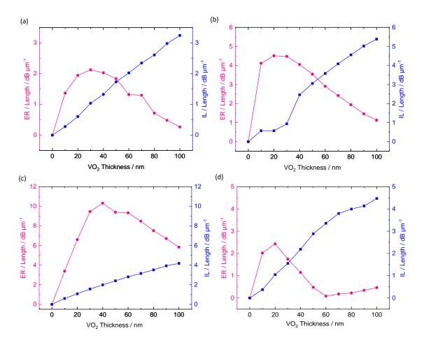
**Figure 7.8:** Simulated extinction ratio ER and insertion loss IL per length  $l_{VO2}$  for (a) the TE mode in device type 1, (b) the TM mode in device type 1, (c) the TE mode in device type 2 and (d) the TM mode in device type 2.
