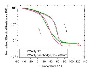
**Figure 6.9:** Electrical characteristics of a VMoO<sub>2</sub> free-standing nanobridge with a width of w = 200 nm, a length of  $l = 5 \mu m$  and the unpatterned reference VMoO<sub>2</sub> film, having the same thickness of t = 100 nm. The difference between the electrical resistance changes of the nanobridge and the film D<sub>w</sub> is indicated by the red arrow. The change R/R<sub>max</sub> is increased for the nanobridge compare to the reference film.
