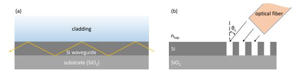
**Figure 3.1:** (a) Schematic illustration of light propagation inside a Si waveguide by total reflection, and (b) Si grating coupler for light coupling from an out-of-plane source by an optical fiber (not to scale).
