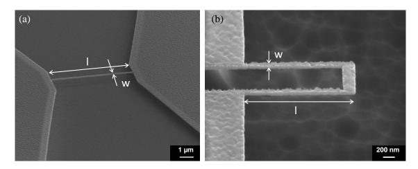
**Figure 5.6:** SEM images of VMoO<sub>2</sub> free-standing structures fabricated by the direct nanomachining of deposited films on SiO<sub>2</sub>/Si substrates. (a) A nanobridge with the lateral width of w = 100 nm and the length of  $l = 5 \mu m$ . (b) A Double-beam structure with w = 100 nm and  $l = 2 \mu m$ .
