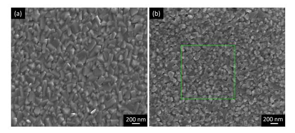
**Figure 5.2:** Scanning electron micrographs of as-deposited films on SiO<sub>2</sub>/Si substrates. (a) A VO<sub>2</sub> film with a grain size of  $125 \pm 5$  nm, and (b) a VMoO<sub>2</sub> film with a grain size of  $100 \pm 5$  nm. The green square indicates a randomly chosen area of  $1.5 \ \mu m \times 1.5 \ \mu m$ , within which the averaged grain sizes of films are determined.
