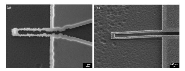
**Figure C.1:** Scanning electron micrographs of nano double-beams fabricated by the direct nanomachining of the VMoO<sub>2</sub> film on a SiO<sub>2</sub>/Si substrate. (a) A structure with rough edges due to incorrect parameters of the EBL process. (b) A collapsed double-beam with a beam width of 200 nm and a length of 6  $\mu$ m, i.e. l/w = 30.
