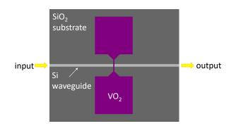
**Figure 7.9:** Schematic of the design of type 2 devices with integrated large pads (0.5 x  $0.5 \mu m^2$ ) for electrical connections.
