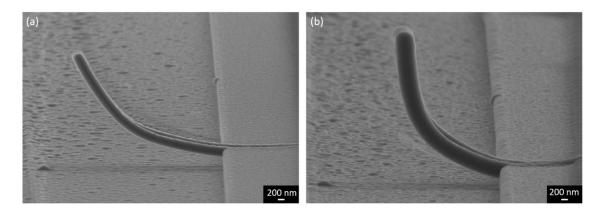
**Figure 6.15:** SEM micrographs of a Cr/VMoO<sub>2</sub> double-beam actuator with w = 300 nm and  $l = 6 \mu m$  at the temperature of 85 °C, (a) before starting the measurement, and (b) after three cooling-heating cycles. The focus window of the SEM and the magnification is kept fixed over the entire measurement of exceeding 6 hours. The morphology of the film surface and the double-beam is changed. A thickening effect is observed.
