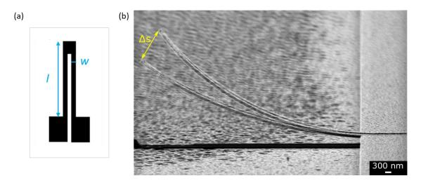
**Figure 6.12:** (a) Top-view schematic of a double-beam nanoactuator with the width of w and the length of l. (b) Overlay of two SEM images of a Cr/VMoO<sub>2</sub> double-beam actuator with  $l = 12 \mu m$  and w = 600 nm at temperatures of -40 °C and 85 °C. Thickness of Cr and VMoO<sub>2</sub> films are 37 and 100 nm, respectively. An upward deflection  $\Delta s$  is observed upon cooling under quasi-stationary conditions.
