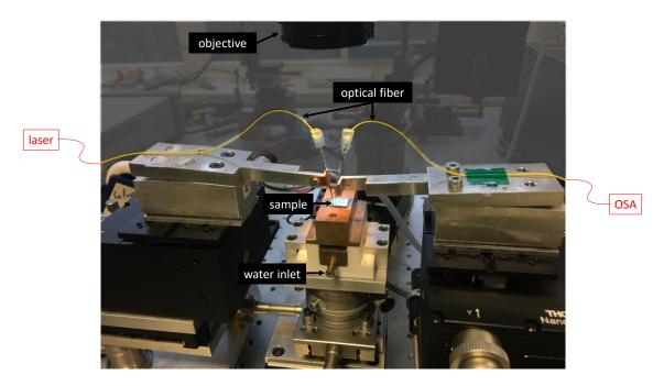
**Figure 7.13:** Optical setup for transmission measurements. Laser light is coupled by an optical fiber through a grating coupler into the waveguide. The transmitted light is coupled out to a fiber through a second grating coupler. The intensity is measured by an optical spectrum analyzer. The sample is placed on a rotational stage. Inlet and outlet ports allow for heating/cooling by injection of water at different temperatures.
