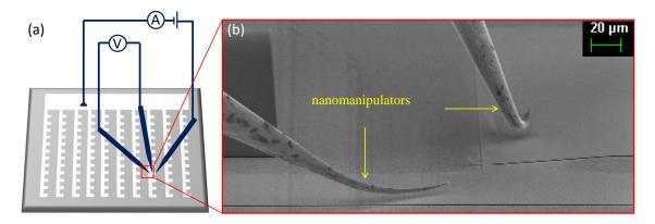
**Figure 6.18:** (a) Schematic of the four-point-probe setup for Joule heating measurements inside a SEM. (b) Scanning electron micrograph of a  $Cr/VMoO_2$  double-beam and two nanomanipulators positioned at each side of the structure to measure the voltage.
