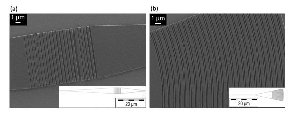
**Figure 7.10:** Scanning electron micrographs of Si grating couplers for out-of-plane light coupling of (a) TE modes and (b) TM modes at the wavelength of 1550 nm.
