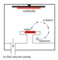
Figure 4.1: Sketch of a typical electron beam physical vapor deposition (EBPVD) system.
