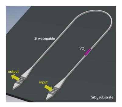
**Figure 7.2:** Schematic of design concept of a photonic switching device using the metal-insulator transition of a VO<sub>2</sub> film covering a section of a Si waveguide. The input optical power either propagates through the waveguide to the output for the VO<sub>2</sub> film in insulator state or absorbed by the VO<sub>2</sub> film in metal state.
