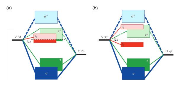
**Figure 2.5:** Schematic depiction of the  $VO_2$  band diagram based on the Goodenough's model for (a) the rutile R crystal structure corresponding to the metal state and (b) the monoclinic M1 structure of the insulator state. The Fermi level is indicated by  $E_F$ . Adapted from [82].
