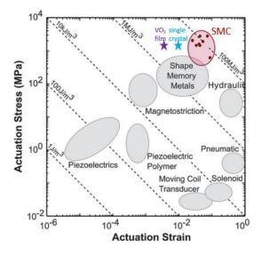
**Figure 2.4:** Comparison of actuation stress and strain diagram for various materials and systems. Dashed lines indicate contours of equal work output densities. Shape memory ceramics (SMC) offer work output values approaching 100 MJ/m<sup>3</sup>. Stars indicate work outputs of VO<sub>2</sub> films and single crystals exceeding 10 MJ/m<sup>3</sup>. Adapted from [45].
