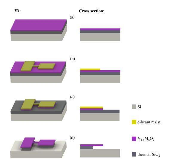
**Figure 5.5:** Schematic of the fabrication flow of the direct nanomachining of as-deposited  $V_{1-x}M_xO_2$  films. After (a) reactive magnetron sputtering of the  $V_{1-x}M_xO_2$  film on the SiO<sub>2</sub>/Si substrate, (b) patterns of structures, here nanobridges, are transferred to the resist by the e-beam lithography. (c)  $V_{1-x}M_xO_2$  film is etched by the RIE. (d) Undercut of the thermal SiO<sub>2</sub> by the fluidic HF acid creates free-standing structures.
