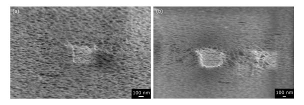
**Figure 6.16:** SEM micrographs of VMoO<sub>2</sub> films after temperature-dependent measurements. The surface of the film after 10 min of exposure to the SEM e-beam through a reduced scanning window at 25 °C. (a) and at -35 °C (b) indicating local change of crystal structure. Reduced scanning windows can be recognized by the brighter rectangular areas in the middle of graphs.
