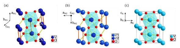
**Figure 2.3:** Schematic depiction of VO<sub>2</sub> crystal structures for the (a) monoclinic M1 phase at  $T < T_{tr}$ , (b) the monoclinic M2 phase at  $T < T_{tr}$  and (c) the tetragonal R phase at  $T > T_{tr}$ . Adapted from [62].
