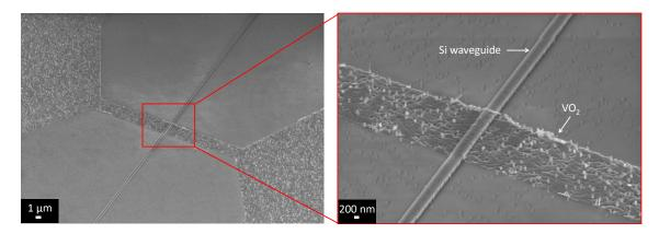
**Figure 7.12:** Scanning electron micrographs of a fabricated type 2 device with large pads for electrical connections. The thickness of the  $VO_2$  film is 60 nm. Small cylinders distributed on the substrate are black silica structures that are produced by cryogenic Si etching, due to slight fluctuations of etching parameters inside RIE chamber.
