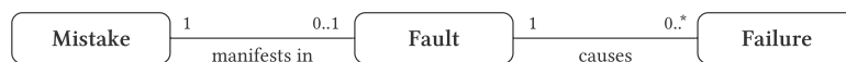
Figure 2.3.: UML representation of the concept of a causal chain between a mistake, a fault, and several failures.
