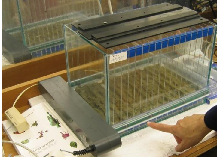
Figure 2.1: Activity monitor for T. saltator . When animals emerge above sand level they break an infra-red which was recorded and processed by a personal computer attached. Photograph taken by Laura Schumm.
