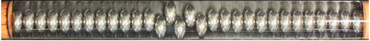
FIG. 7: Buckled chain of 30 steel spheres (diameter 6.32\text{ mm} ) confined in a perspex cylinder (inner cylinder diameter 1.6\text{ cm} ) and under compression, \Delta = 0.85 . The spheres, which are undeformed, are immersed in vegetable oil to reduce friction between them. (The presence of the oil leads to a large optical distortion; the measured ratio of lateral sphere extension to sphere diameter is about 1.9.)
