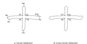
Fig. 5. The detection result of real cross-corners. The Chinese character "Ten" is applied as an example. (a) The detection result of the first process. The cross-corners are labeled P1 to P10. (b) The detection result of the second process. Only Points P2, P4, P7, and P9 are real cross-corners.
