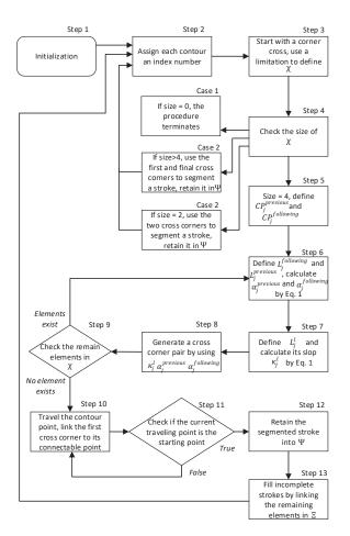
Fig. 7. The flowchart of the stroke decomposition procedure.
