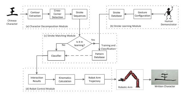
Fig. 3. The architecture of the proposed approach for robotic handwriting. The approach contains four modules: (a) character decomposition module, (b) stroke learning module, (c) stroke matching module, and (d) robotic control module.
